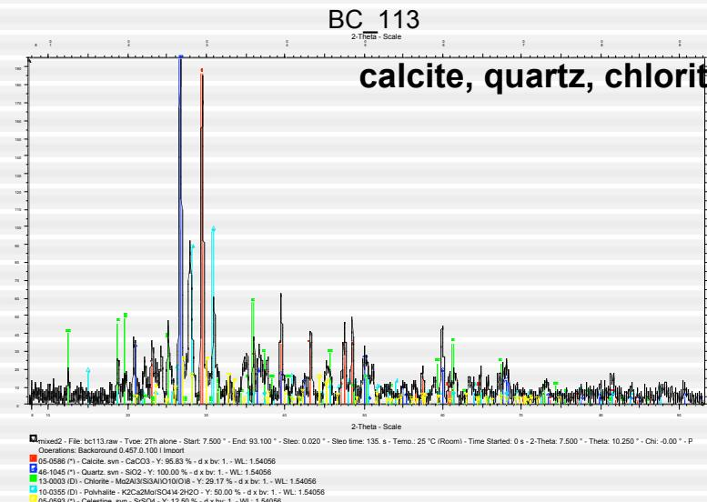
X-Ray diffraction on the sample BC113
