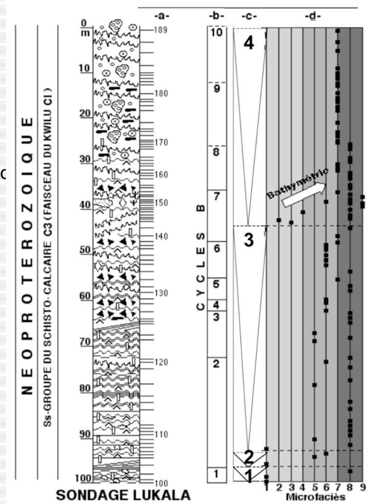
Stratigraphic log of Lukala borehole. Column a = position of analysed samples (petrography), Column b = amalgam of sequences of 4<sup>th</sup> and 5<sup>th</sup> orders, Column c = parasequences of 4<sup>th</sup> order, Column d = standard sequence of microfacies 1 to 9. The arrow corresponds to the bathymetric evolution
