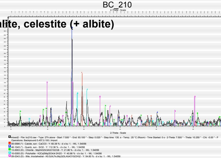
X-Ray diffraction on the sample BC210
